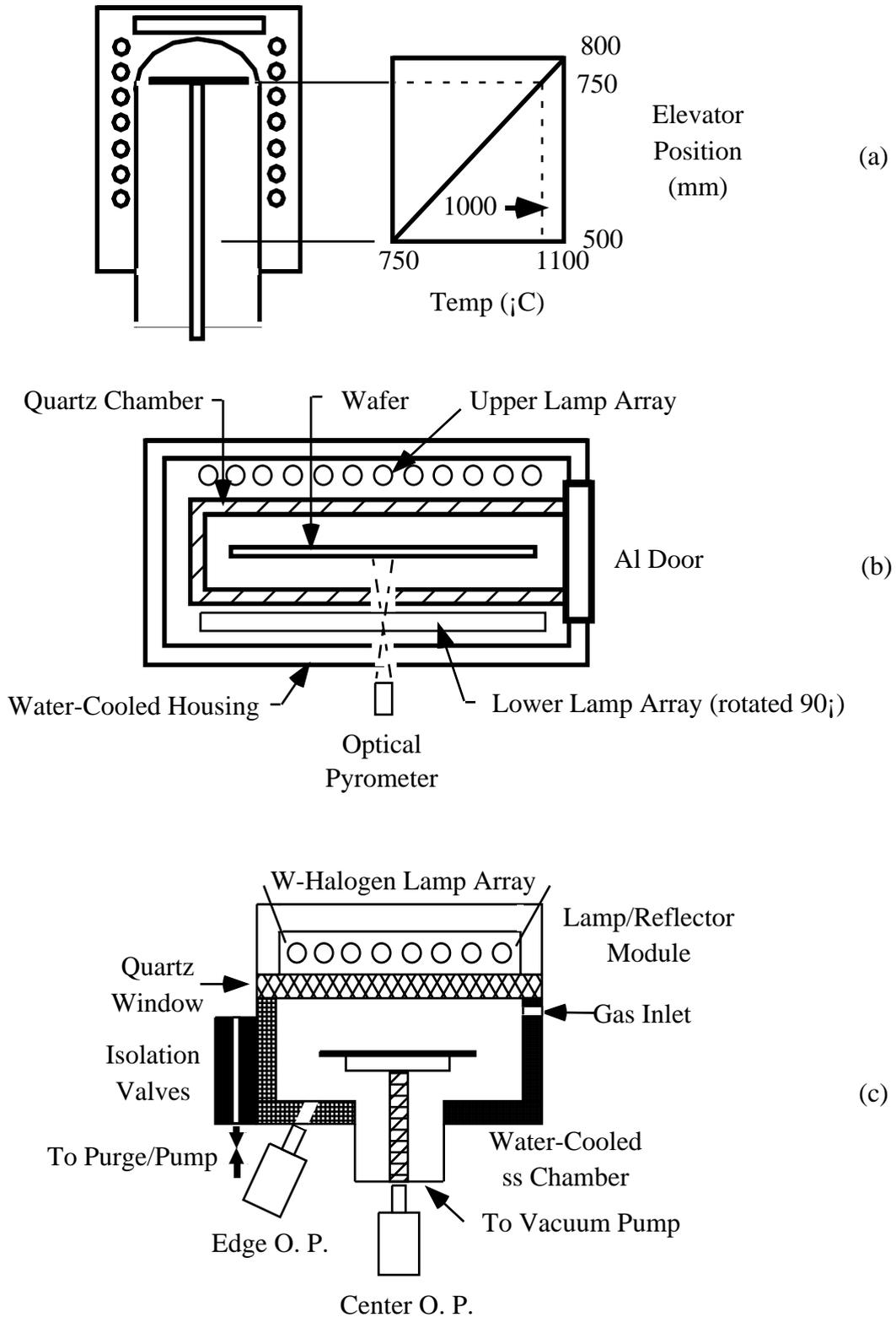
Figure 1: Examples of three RTP system architectures; (a) hot wall; (b) warm wall; (c) cold wall
