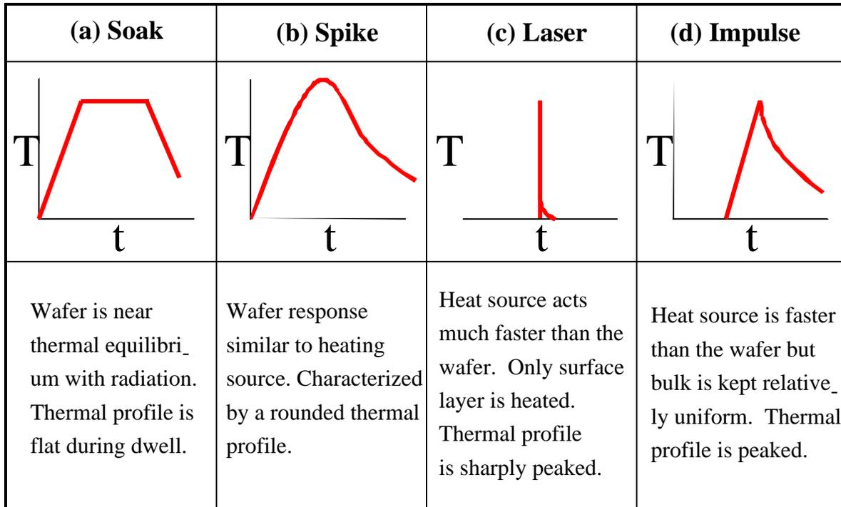
Figure 4: Comparison of four temperature profiles: [21]
